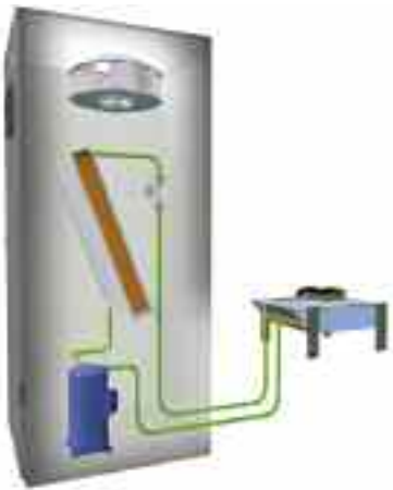
A - Air-cooled with remote condenser
