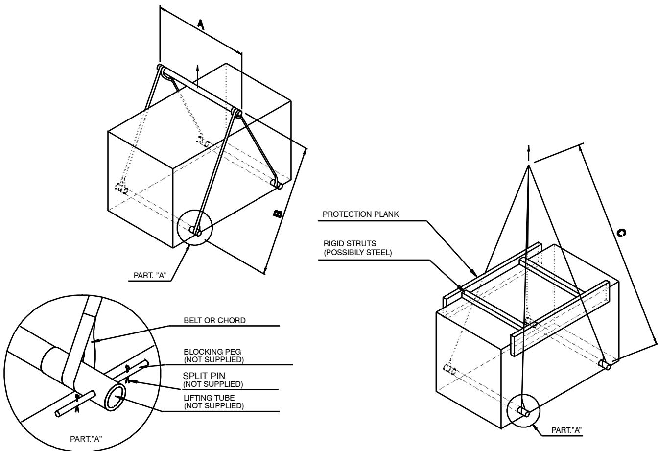
**N.B:** Place the lifting tubes in the holes in the base indicated by the word 'LIFT HERE'. Lock the ends of the tubes in position with the locking pins and split pins as shown above.
