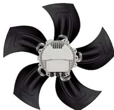
A general noise reduction is further obtained, as the EC technology used for the adjustment does not cause magnetic vibrations, not even on special frequencies corresponding to certain rotation speeds. Finally, the decrease of inrush current thanks to the EC technology and the absence of sliding contacts for the rotor supply significantly reduce the stresses that negatively influence the component life, increasing the machine overall reliability.
