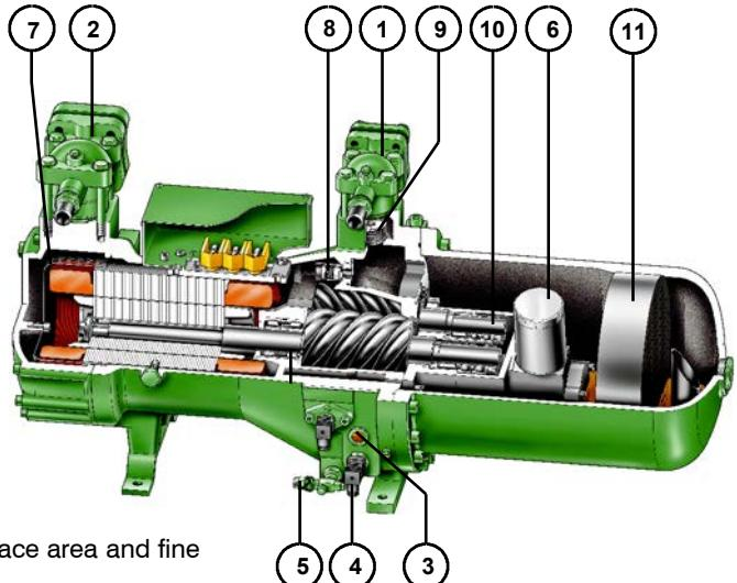
Each compressor is equipped with a three-phase asynchronous two-pole motor located on the shaft of the male screw rotor and cooled by the suction gas. It is removable for inspection and maintenance. The motor start with reduced load is star/delta type.
