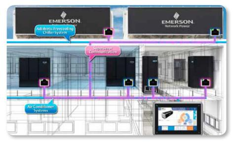
When considering the entire data center scenario, involving indoor and outdoor units, the Supersaver becomes the key driver in terms of delivered efficiency at the data center system level.
