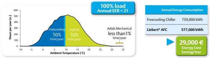
The advantages of the adiabatic and hybrid designs are even more effective at partial load, where the compressor operation throughout the year is further minimized.
