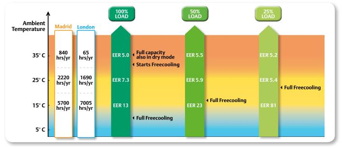
EER values for the FAO Range at the following conditions: adiabatic function active (wet pads mode) and calculated according to the average humidity data obtained from Central Europe locations.
