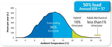
Annual Energy ConsumptionFreecooling Chiller281,000 kWhLiebert® AFC185,000 kWhLiebert® AFC<br/>with Supersaver107,000 kWhLiebert® AFC<br/>with Supersaver107,000 kWh
