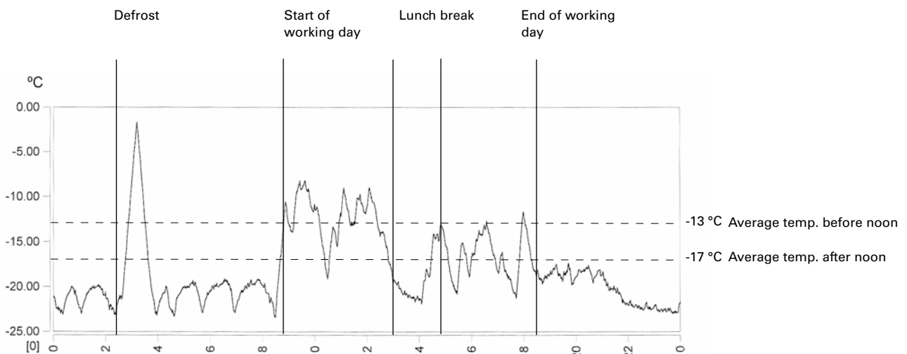
Temperature rise over a 24 hour period using ADA Cool
