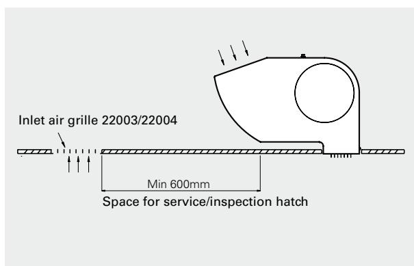
Fig. 2: False ceiling mounting
