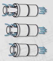
Within the operating pressure differential range, the effective open orifice area of the cartridge is automatically adjusted to the point where the specified flow rate will be delivered (as the pressure differential increases, the open area closes and as it decreases, the area opens).
