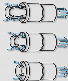
Within operating pressure differential range, the effective open orifice area of the cartridge is automatically adjusted to the point where the specified flow rate will be delivered (as the pressure differential increases, the open area closes and as it decreases, the area opens).
