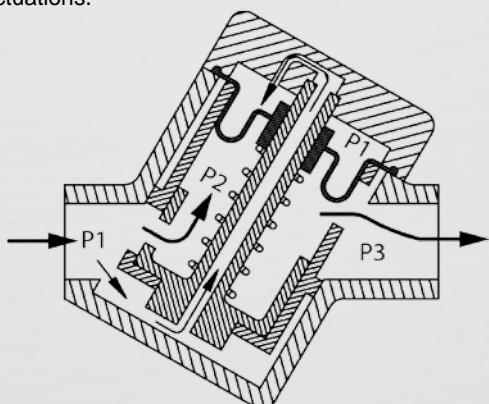
Below its pressure differential range, the valve acts as a fixed orifice. This allows a temperature control valve in the same circuit to operate with valve authority up to the set flow rate maximum.
