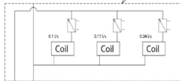
Each branch is automatically balanced due to the correct balance of each coil. Sum total of 0.31 l/sec (branch).
