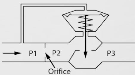
For the FlowCon A/AB/ABV, the principle of operation is shown above and the principle of construction is shown below. P1 and P3 are system pressures, P1-P3 is the total pressure drop across the valve. P2 is set by the diaphragm acting in reaction to P1 in the upper diaphragm chamber. Interacting with the spring, P1-P2 remains constant, keeping a constant  $\Delta P$  across the orifice areas. The result is a constant flow rate through the valve, independent of pressure fluctuations.
