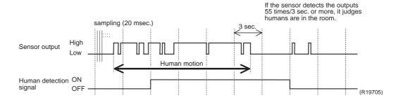
The sensor detects human motion by receiving infrared rays and displays the pulse wave output.
