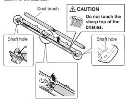
Confirm that the dust brush is securely attached. Otherwise, the dust brush may not rotate and the CLEANING FILTER operation may not be performed.
