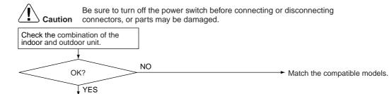
Check the code numbers (2P012345, for example) of the indoor and outdoor unit PCB with the Parts List.
