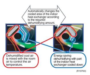
Energy saving dehumidifying is realised by cooling down the part of the indoor heat exchanger. Dehumidified cool air is mixed with the room air to be near room temperature and blown into the room. The area of indoor heat exchanger used for dehumidifying is automatically controlled according to the required dehumidifying amount. The larger/smaller the required dehumidifying amount, the larger/smaller the heat exchange area.
