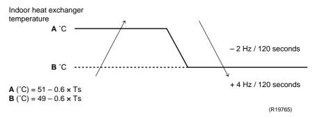
Also, the followings are controlled in order to improve energy efficiency, considering room thermistor temperature, set temperature, and airflow rate.
