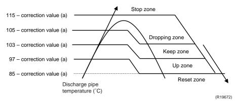
Correction value (a) = correction value by operation frequency (b) + correction value by outdoor temperature (c)
