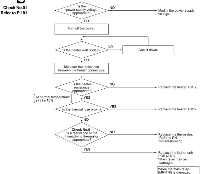
heater and rotor do not run.
