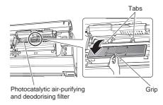
Attaching the photocatalytic air-purifying and deodorising filter
