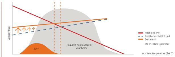
Compared to a traditional On/Off unit, the requirement for support from the back up heater is much lower for the Daikin Altherma ground source heat pump, thanks to the boosting effect of our inverter compressors, also this leads to lower running costs.
