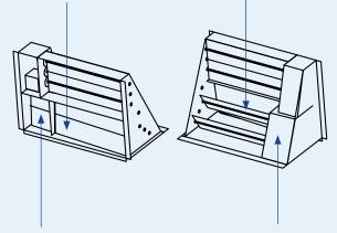
New enclosed space within economizer isolates the 1st stage relief damper from the effects of the indoor fan. The damper always relieves air in direct relation to the building pressure.
