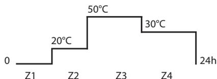
The "daily" and "variable set point" time bands can be programmed to set steam production according to the requirements of the operator of the steam bath (e.g. based on closing times) and with a customised temperature trend (using the 4 set point threshold).
