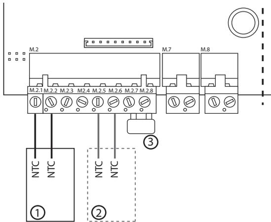
Fig. 4.e (detail of electronic board, humidifier electrical compartment)
