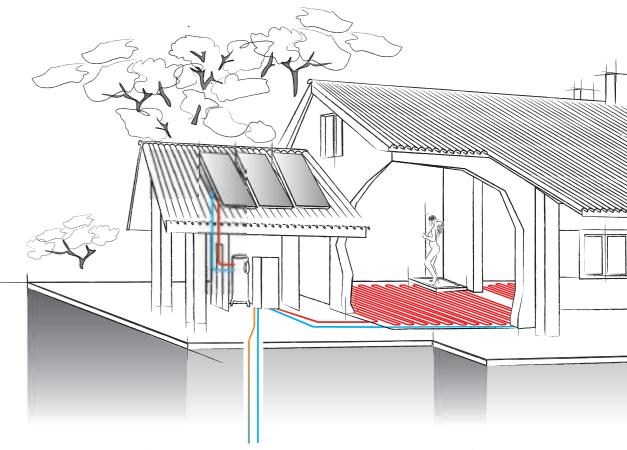
Following years of success in air-conditioning controllers, CAREL offers the first complete integrated electronic solution for managing ground source heat pumps, for residential applications and swimming pools, ensuring energy savings and optimising the management of the entire system. Within the many possible applications, CAREL guarantees a range of solutions that can adapt to the growing levels of integration between the heat generator and the system.
