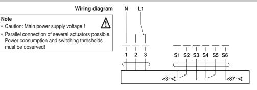
Actuator for smoke control dampers 90  $^{\circ}{\triangleleft},$  AC 230 V, 15 Nm
