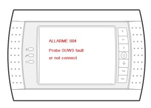
The value read by the SUW3 probe is out of range -35°C / 80°C independently if it is connected to the PCO1 or PCOE card
