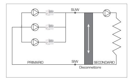
The power of the chillers switched-on is calculated with this system, taking into consideration the temperature differential between SIW and SUW compared with the chiller full load Delta parameter that represents the DT between evaporator water input and output of a chiller at full power (parameter to be set in the basis of the project conditions). In this way, the choke level of the chillers switched-on is evaluated (% LOAD).
