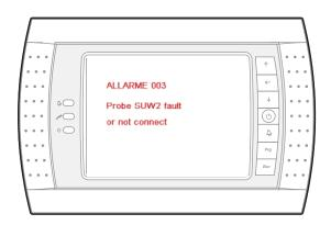
The value read by the SUW2 probe is out of range  $-35^{\circ}$ C /  $80^{\circ}$ C independently if it is connected to the PCO1 or PCOE card
