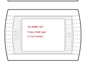
Il The value read by the SUW probe is out of range  $-35^{\circ}$ C /  $80^{\circ}$ C independently if it is connected to the PCO1 or PCOE card
