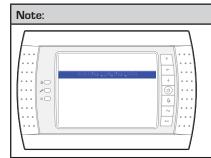
By pressing the icon key of each chiller, access the visualisation menu of the details of the relative chiller. This page appears for a few seconds during loading of the data if the chiller is present. If the chiller is not present (the icon of a blue square is pressed) this page remains indefinitively.
