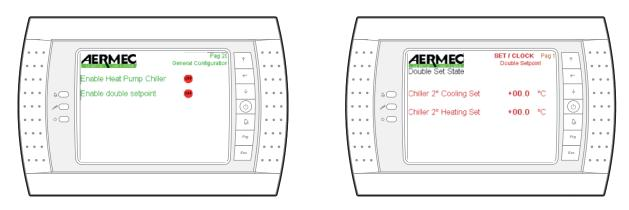
By enabling the double set point function (**Enable double set point**) by means of a contact that is not live, connected to the digital input ID3, it is possible to decide whether to use the normal set points or double set alternatively (e.g. night-time functioning).
