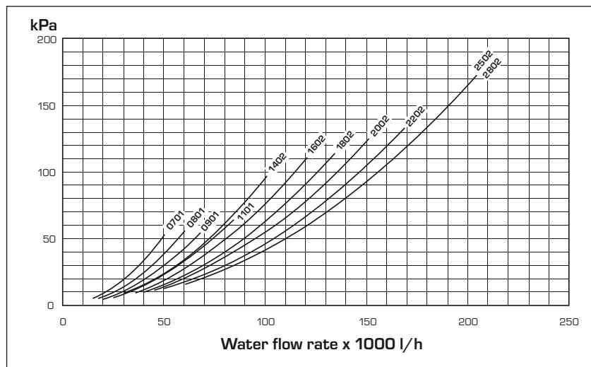
The pressure drops in the diagram refer to the average water temperature of 10 °C: the following table shows the correction to be applied to the pressure drops when the average water temperature varies.
