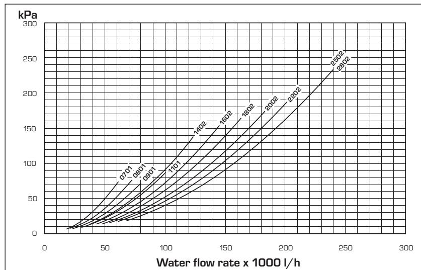
The pressure drops in the diagram refer to the average water temperature of 30 °C: the following table shows the correction to be applied to the pressure drops when the average water temperature varies.
