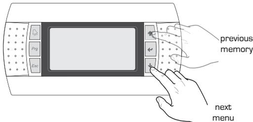
(c) When the desired menu is displayed, press the
