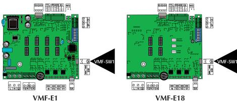
The diagrams represent the thermostat circuit boards. Probe connection and Dip-Switch setting
