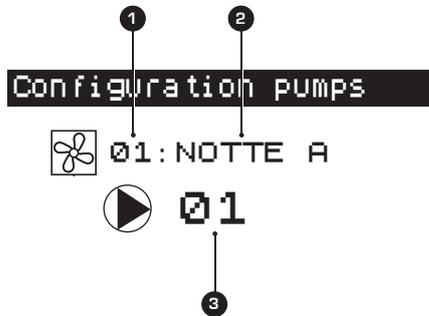
To manage activation of the pumps, they must be associated to the master fan coils of the zone they serve; this window displays the following information:
