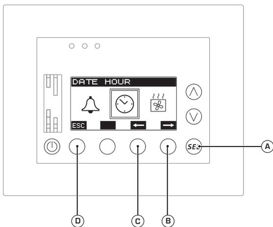
On the menu selection page, the icon inside the frame represents the selectable submenu (the identification string is provided at the top left). At this moment the possible operations are:
