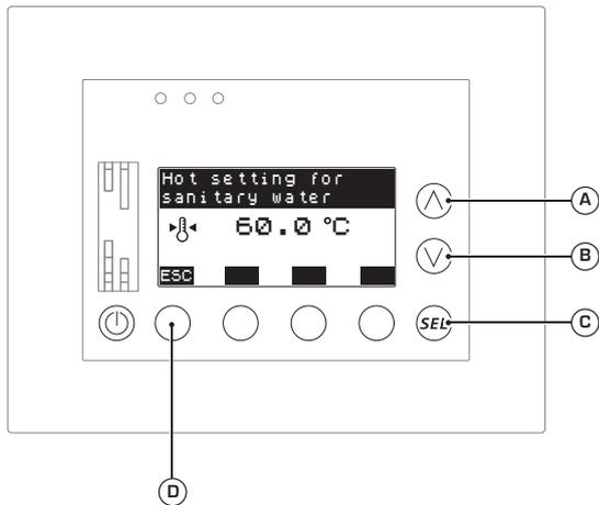
When the system demands domestic hot water, the unit will produce hot water at the temperature indicated in this parameter (the value can be between 30.0 and 70.0°C); to set this value it is necessary to:
