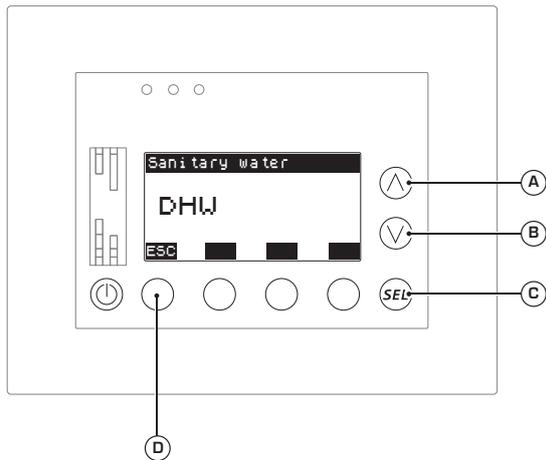
The presence of the VMF-ACS accessory in the system is the fundamental requirement to allow production of domestic hot water. This parameter specifies whether this accessory is present in the system; to set this value, it is necessary to:
