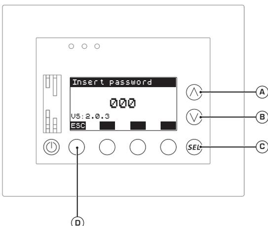
The first window of the ASSISTANCE menu allows the installer to access the menu by entering a three digit password; to set this password, it is necessary to:
