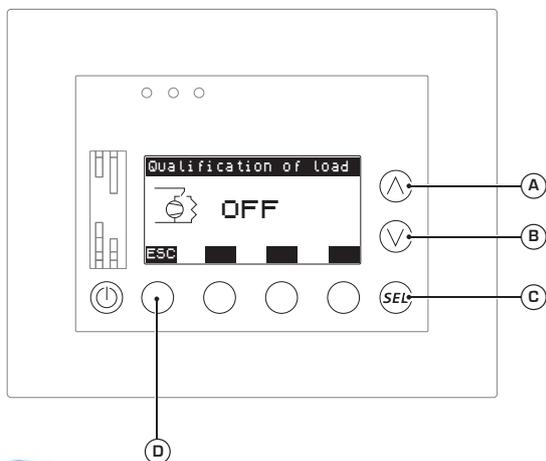
This parameter specifies whether the system allows simultaneous activation of chiller loads (compressor plus possible supplementary electric resistance inside the chiller) and those linked to domestic hot water (electric resistance in DHW storage tank); to set this value it is necessary to:
