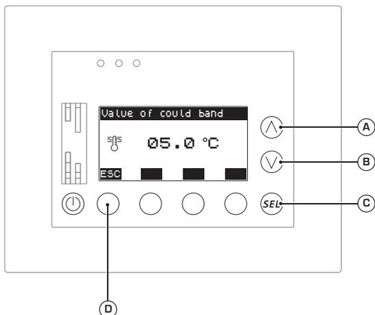
In VMF systems, if the user sets the Economy mode, the cooling work setting will vary dynamically based on the actual thermal load required by the system (maximizing energy-saving); the variation of the cooling work setting is included in a band which goes from the work setting to the same setting minus the value specified in this parameter (the value of this parameter can be from 3.0 to 20.0°C); to set this value it is necessary to:
