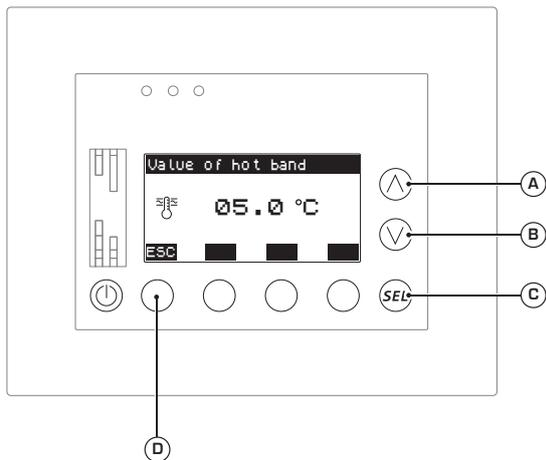
In VMF systems, if the user sets the Economy mode, the heating work setting will vary dynamically based on the actual thermal load required by the system (maximizing energy-saving); the variation of the heating work setting is included in a band which goes from the work setting to the same setting minus the value specified in this parameter (the value of this parameter can be from 3.0 to 20.0°C); to set this value it is necessary to:
