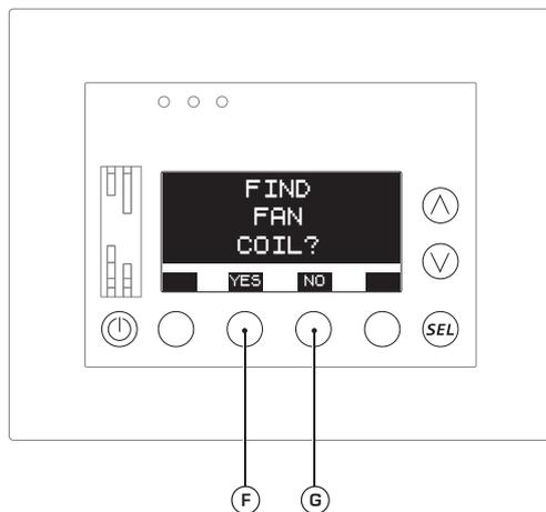
The VMF-E5 control panel implements the self-detection procedure which allows each thermostat connected to the MASTER fan coils to automatically be assigned with a univocal address. In order to activate this procedure it is necessary to:
