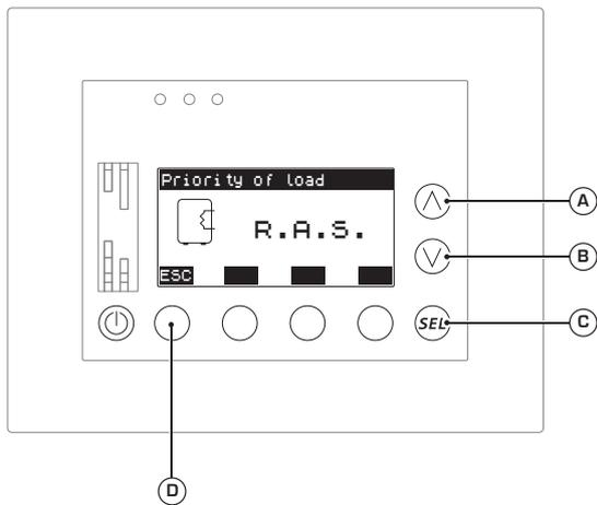
The VMF systems can have installations with two electric resistances, one on the heat pump and another in the DHW storage tank; this function allows to establish which of these resistances is used during domestic hot water production; to set this value, it is necessary to:
