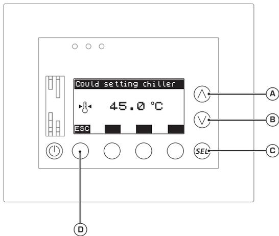
In summer, the user will set the desired room air temperature by means of the thermostat on the master fan coils. To reach this temperature, the unit will produce cold water at the temperature set by the installer indicated in this parameter (between 00.0 and 20.0°C); to set this value it is necessary to:
