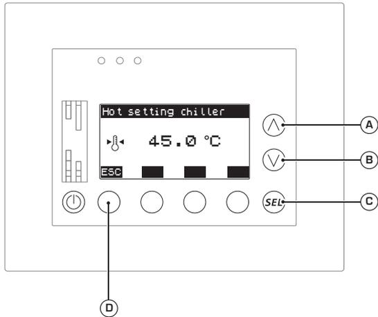
In winter, the user will set the desired room air temperature by means of the thermostat on the master fan coils. To reach this temperature, the unit will produce hot water at the temperature set by the installer indicated in this parameter (between 30.0 and 70.0°C); to set this value it is necessary to:
