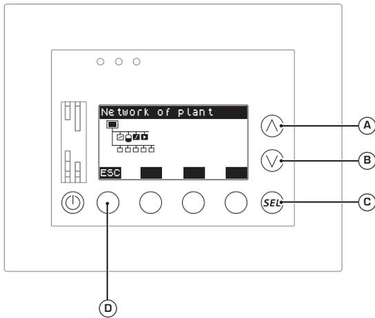
This window indicates the graphic resulting from all parts connected to the VMF system; the diagram is created dynamically and represents the status of the serial communications between the VMF-E5 accessory and the other parts of the system; the symbols displayed in the graphic are arranged in several rows; the first can include (from left to right):
