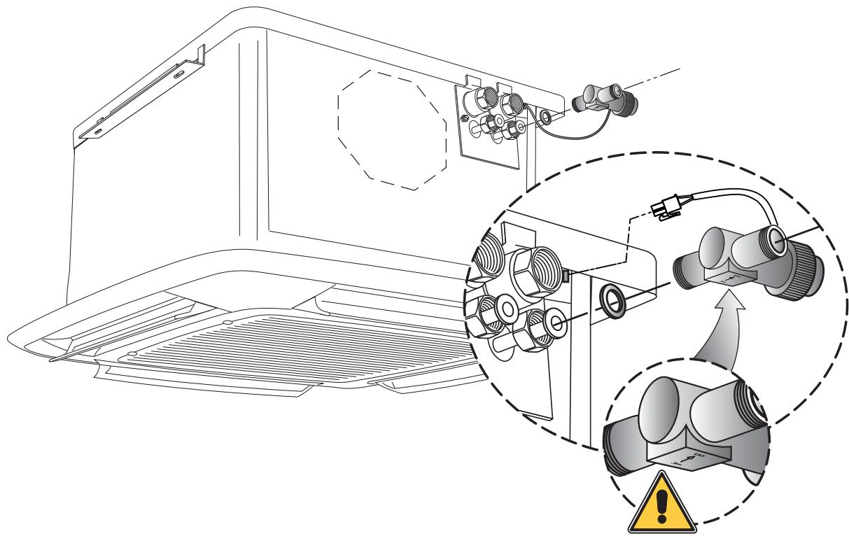
**UK** The kit is composed of a valve, the relative actuator and one gasket.
