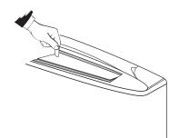
Ventilation is only allowed with the fin open; it must be manually opened.
