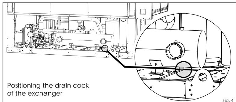
Positioning the drain cock of the exchanger
