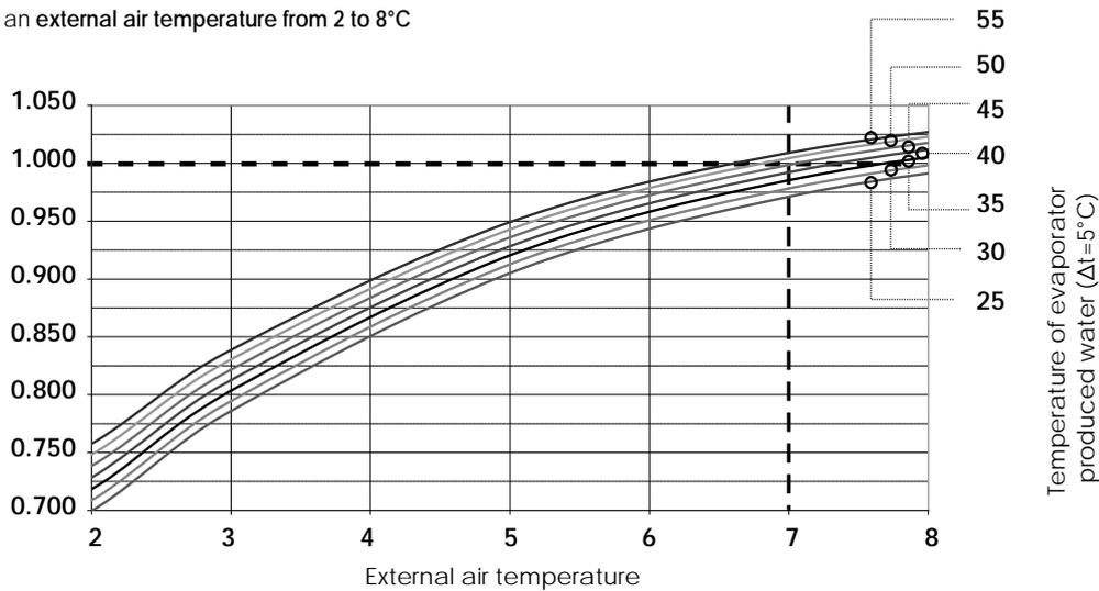
Corrective coefficients (Ca) of the input power (Pe)
