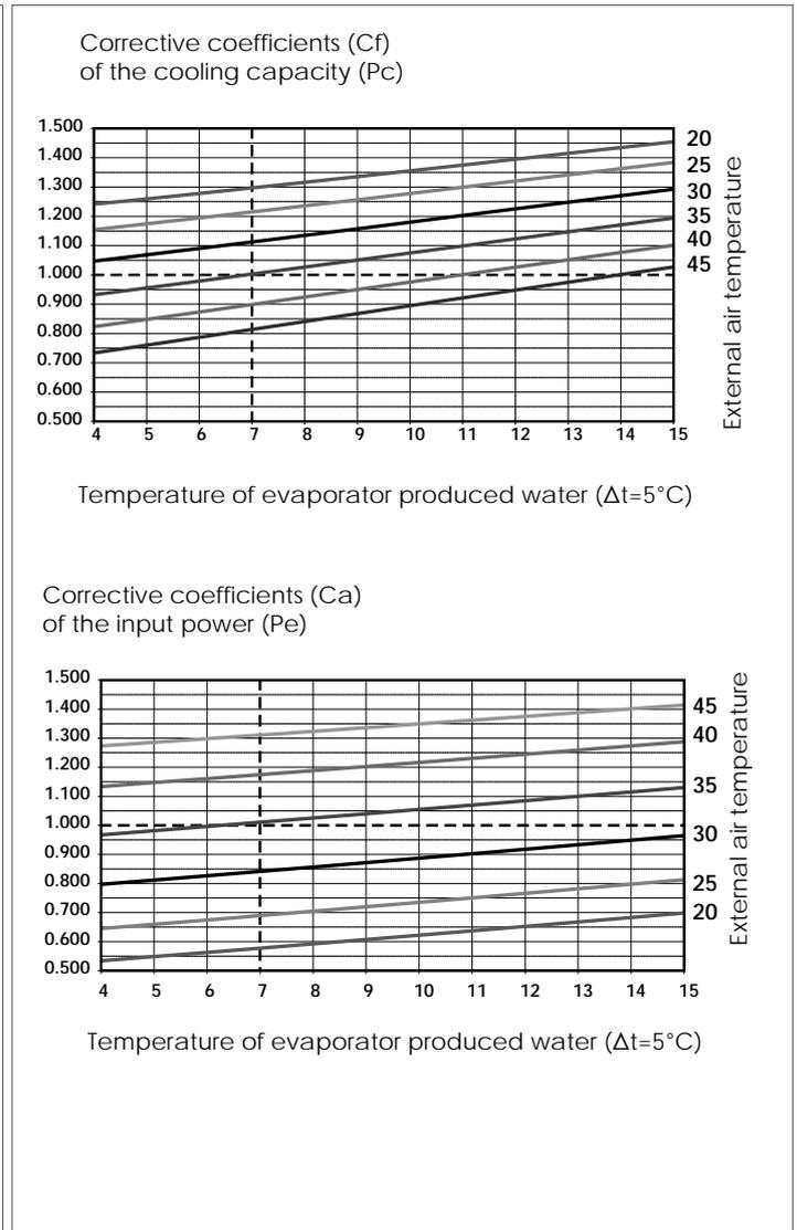
The cooling capacity and electrical input power in conditions other than normal conditions are obtained by multiplying the nominal values of the Pc and Pe (see technical data) by the respective coefficient correctives (Cf, Ca).
