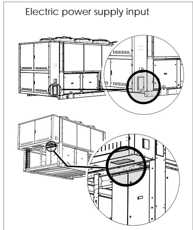
For longer lengths or different cable laying, it is up to the PLANNER to calculate the appropriate line switch, the power supply line as well as the connection to the earth wire and connection cables depending on:
