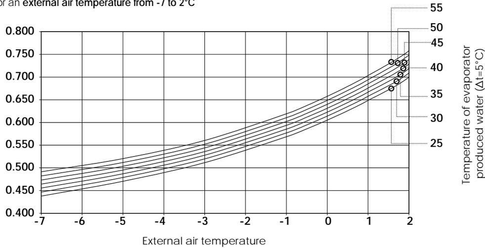
Corrective coefficients (Ca) of the input power (Pe)
