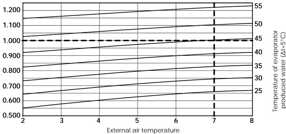
The heating capacity and electrical input power in conditions other than normal conditions are obtained by multiplying the nominal values of the Ph and Pe (see technical data) by the respective coefficient correctives (Ct, Ca).
