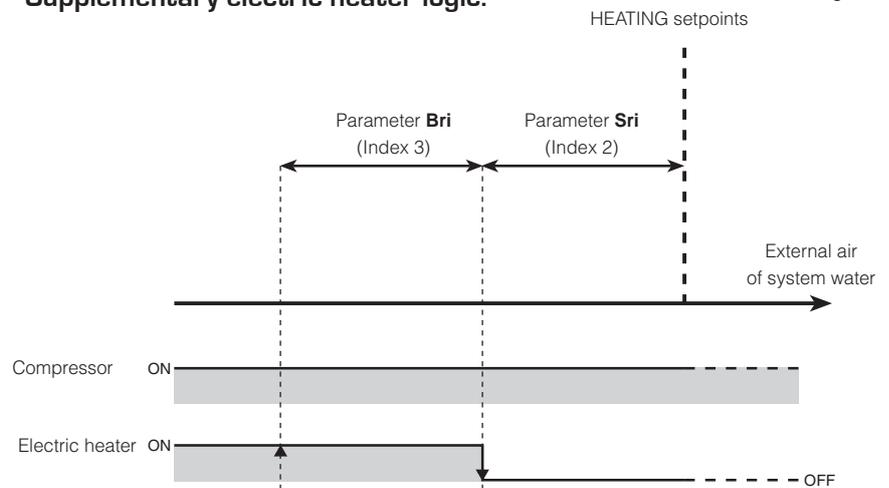
**Replacement electric heater logic:**
