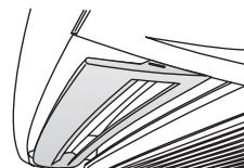
When the fins are closed ventilation is permitted.
