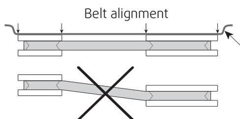
For a quick check, make sure that the small rope touch each end of the pulleys as shown on drawing above.
