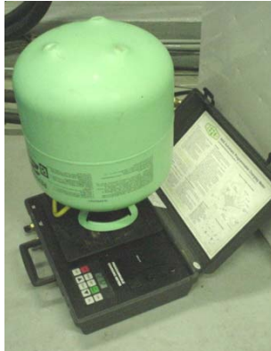
Charging Cylinder on Scale
